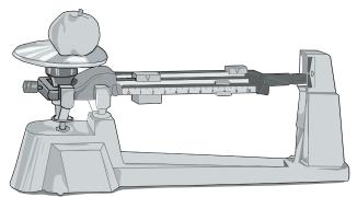
In this activity, you will measure the mass of several different objects using a triple beam balance.
